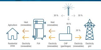
Meeting the grid operator's specification to reduce electrical supply to 30% of CHP nominal capacity due to grid overload: The CHP has to be reduced to only 60% of nominal capacity (less material stress); the P<sub>2</sub>H heater converts the excess electrical power to heat. Result: Both 90% of the heat supply and the requirement for 30% maximum grid supply are met.
