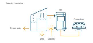
Seawater desalination and simultaneous provision of hot water without a grid connection using renewable energy sources. For example, approx. 15 liters of drinking water per day per m<sup>2</sup> of PV in southern regions. In addition: drinking water treatment in general, thermal recharging of shallow geothermal storage units via PV in the summer.
