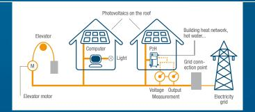
Short-term reduction of heating output when switching on large motors inrush current and avoidance of expanding the grid supply line (service charges, building cost subsidy) when installing renewable energy sources. In addition: excess voltage/wave filtering, balancing of asymmetric load, process heat supply based on available residual grid capacity (process heat for oil or water, for biomass heating return temperature increase).
