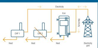
Avoidance of switching on another CHP (or another heat pump) in case of slight heat demand increase in a cascade array. This prevents inefficiency due to double partial-load operation, which also results in higher operating hours. Instead, the ELWA P<sub>2</sub>H system provides the required residual heat generation heat, if necessary using CHP power. In addition: peak time heating and emergency heating.
