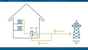
The ELWA P<sub>2</sub>H system can be used as a backup heating system to increase supply security, in particular with heating systems that have moving parts (due to malfunction, maintenance if pellets, oil or a heat pump is used) or in case of a district heating supply. Optimization of plant size and avoidance of a peak time gas heater (base fee, maintenance, chimney sweep). In addition: supplemental revenue from control energy or from not remunerated excess power.
