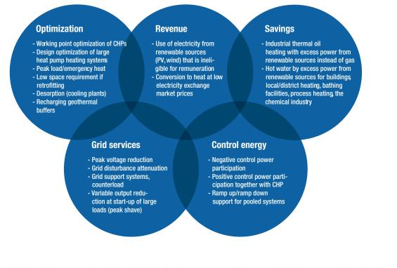
Other application advantages: ahead-of-schedule legionella treatment with excess electrical power, recharging of shallow geothermal energy buffers, reduction of primary energy factor Pf with district heating supply, return temperature increase at biomass heating, supporting variable power ability of biomass powerstations, counter-load for black start generators.
