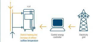
Intake of control energy (primary/secondary control power, minute reserve power as necessary) and reasonable energy use by transferring it to the heating grid. Grid relief, reduction of fossil-based power consumption, increase in maintenance interval length for the main heat source, support at pooled ramp-up and down. In addition, positive control power can be offered by switching off the ELWA P<sub>2</sub>H system on request during the offer period.
