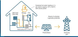
With heating systems that use heat pumps or low temperature furnaces, on appropriate days, excess electrical power that is not eligible for remuneration can be used at midday to provide ahead-of-schedule Legionella protection in the hot water tank with the ELWA P<sub>2</sub>H system (heating up to 70–75°C (158–167°F). This enables savings due to heating system design optimization with efficient, low water temperatures. In addition: emergency heating / peak load heating.
