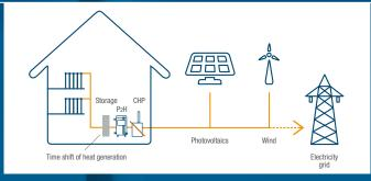
Some electrical power from renewable sources is not eligible for remuneration because otherwise, the power lines would be overloaded. The ELWA P<sub>2</sub>H system transfers the output that the grid cannot accept to the building/local/district heating system. This reduces the use of fossil energy sources. Additionally: supplemental revenue by using electricity from the grid when electricity exchange market prices are low, emergency/peak load heating.
